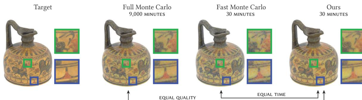
**Figure 1:** We propose a neural scattering compensation for 3D color printing. Comparing to a method which uses noise-free Monte Carlo simulation our technique achieves 300× speedup in the above case while providing the same quality.
