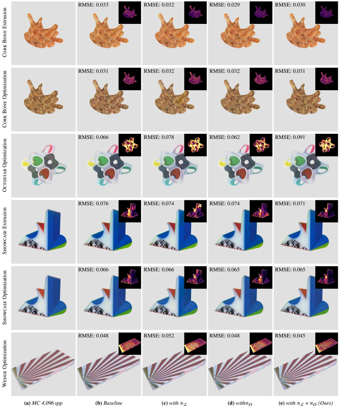
**Figure 12:** Single forward predictions comparing four architecture variants over prediction error (RMSE) for general geometry. The baseline, a basic adaptation of [KMM<sup>\*</sup>17]’s RPNN, is compared against our weight sharing over levels  $\equiv_{\mathcal{L}}$  and octants  $\equiv_{\mathcal{O}}$ . The objects’ unique features are discussed in Section 5. CIE dE 2000: 0 10
