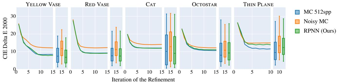
**Figure 8:** Convergence plots for the five fabricated objects in Figure 9 using three prediction methods: MC-based refinement with 512 spp, our network-based solution and an equal-time MC prediction. Average CIE dE 2000 metric values against the target object are derived from a reference MC (re-)prediction (512 spp) for all methods. Boxplots show the 0.05, 0.25, 0.5, 0.75, and 0.95 quantiles of the last iteration.
