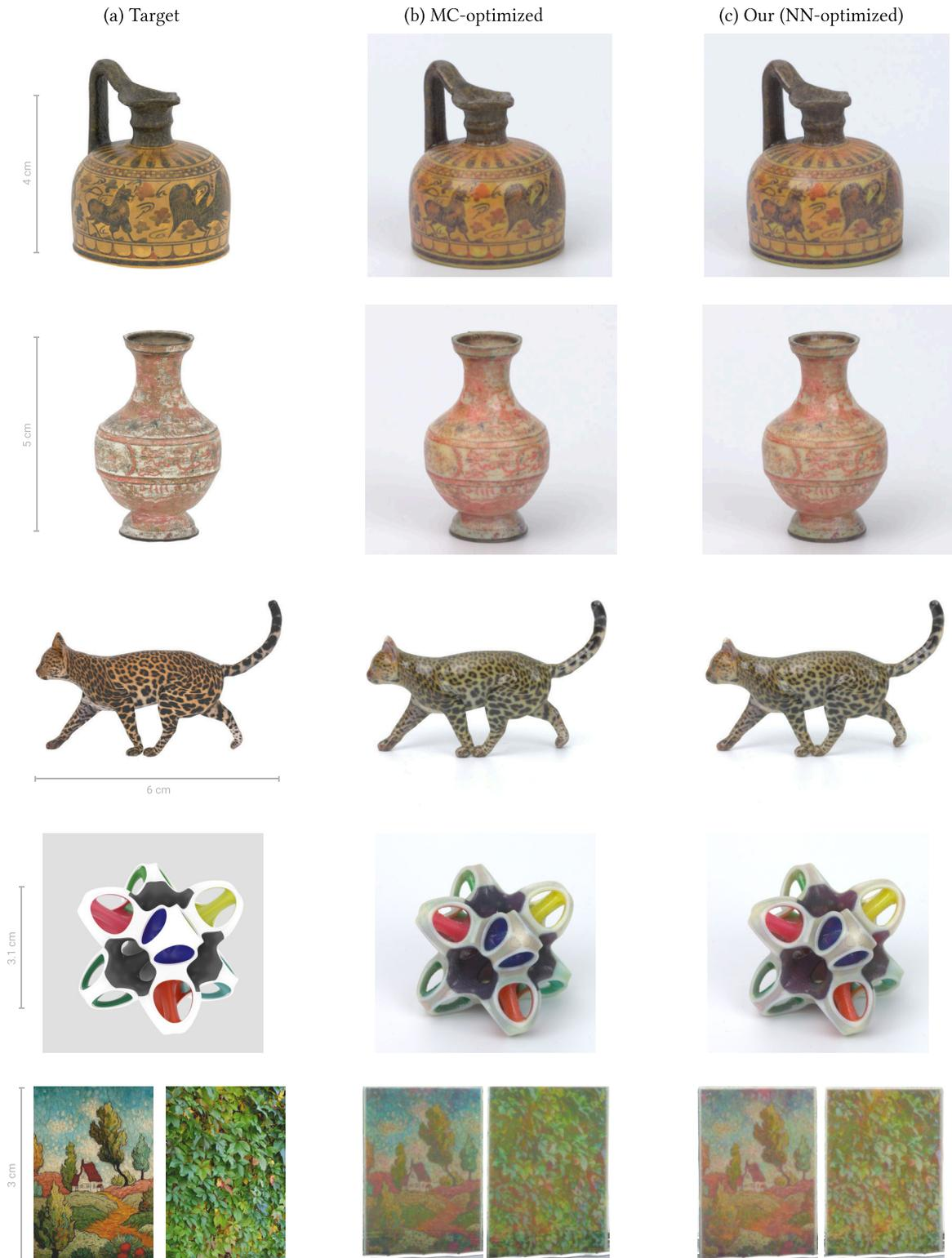
**Figure 10:** Comparison of photographed printouts to the rendered target models (a): refinement solution [SRB\*19] with MC-based predictions (b), our proposed solution with RPNN-based predictions (c). The bottom object is a thin planar slab (0.5 mm thick) with two different textures on its front and back sides.
