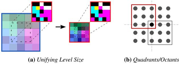
**Figure 6:** Weight sharing. (a) Hierarchy levels are rescaled to the same size (with adjusted optical density) to enable processing with the same weights across levels ( $\equiv_{\mathcal{L}}$ ). (b) On each level, the stencil is split in half per axis and we share weights ( $\equiv_{\mathcal{O}}$ ) over correctly rotated quadrants (octants in three dimensions) to enforce symmetry following from rotational invariance around the black central point  $\mathbf{x}$ .
