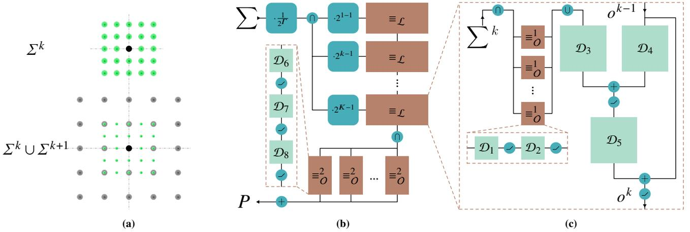
**Figure 5:** Network Architecture: (a) visualizes the spatial relationship between levels inside one stencil  $\Sigma$  and the central point  $\mathbf{x}$ . (b) Network overview where  $\mathcal{D}$  blocks mark dense layers with trainable weights,  $\equiv$  blocks indicate shared weights and round edges/circles signify arithmetic operations ( $\cap$ : slicing,  $\cup$ : concatenation) The factor  $\frac{1}{2^k}$  keeps values in range for training stability. (c) Detail of one RPNN block.
