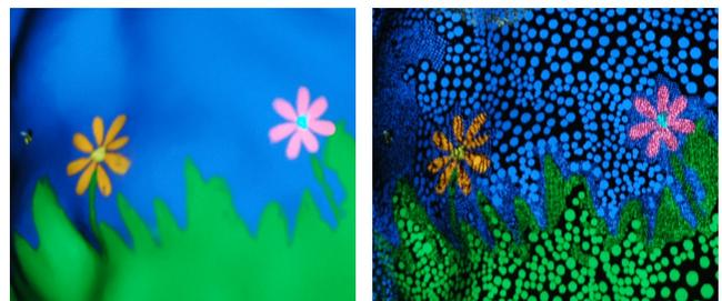
**Figure 11:** ASIC rendering of an irregularly sampled surface. On the right, the splats have been artificially shrunk to illustrate the sample distribution. Images show photographs taken off a screen.
