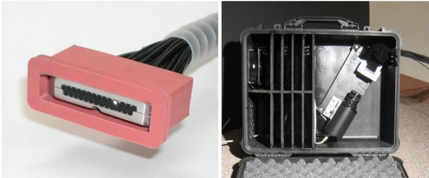
**Figure 8:** Left: A picture of the sensor head with linear fiber array. The source fiber is lit. Right: The fiber array leads to a camera in a light-proof box. The box is cooled to minimize imaging sensor noise.
