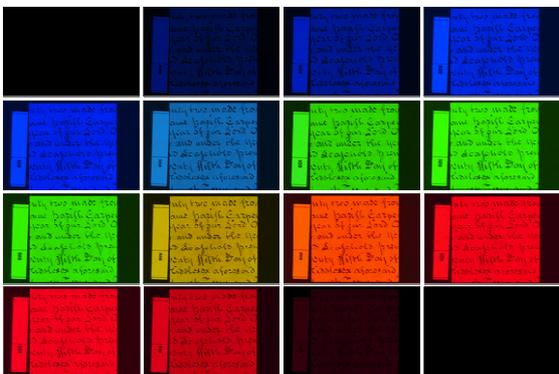
**Figure 6:** Reflective RGB multispectral image set of sample 509 at 16 wavelengths from 400 to 700 nm
