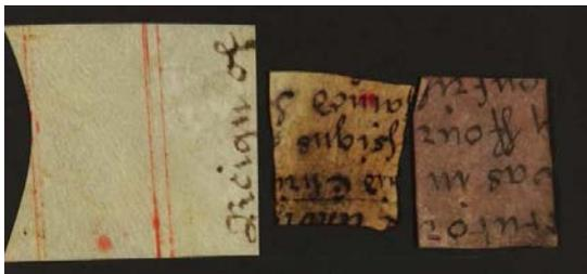
**Figure 11:** Three test samples submitted to soaking in oil, tea and wine, under reflective lighting
