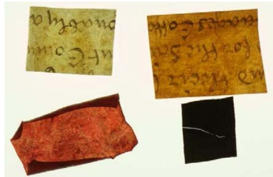
**Figure 12:** Four test samples submitted to desiccation, smoking, soaking in blood and burning, imaged under transmissive lighting
