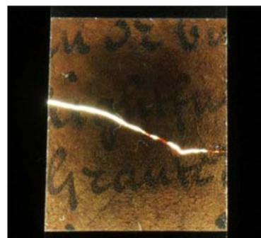
**Figure 14:** A burnt test sample, imaged through transmissive lighting using a very long exposure
